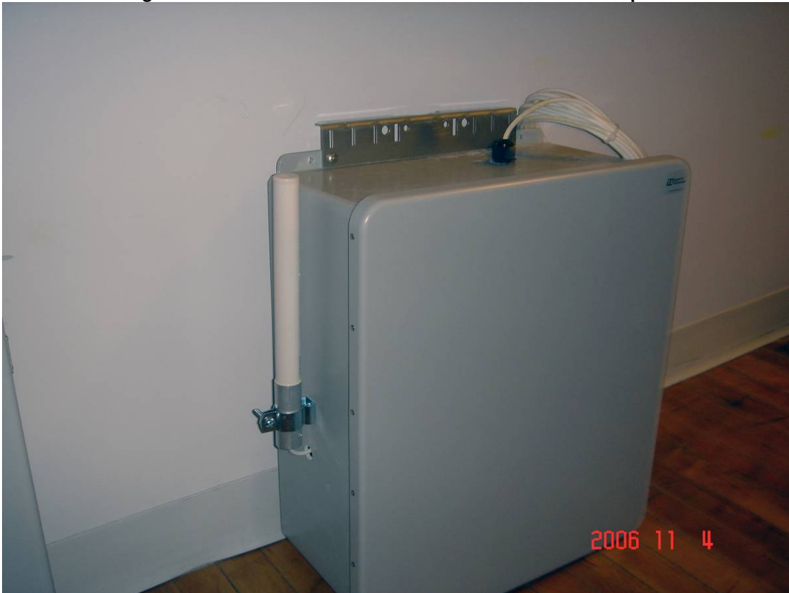
Figure 3: Environmental Enclosure for Outdoor WiFi Hot-spots
